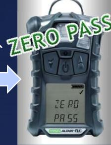
1, Press central button to turn on. Wait for Normal Measure mode.
