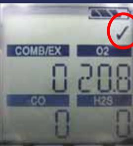
9, The ✓ symbol will be displayed in the Measure mode for 24 hours after a successful Calibration.
