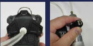
7, Connect tube with the cylinder regulator. Open the pressure reducer valve on test gas cylinder.
