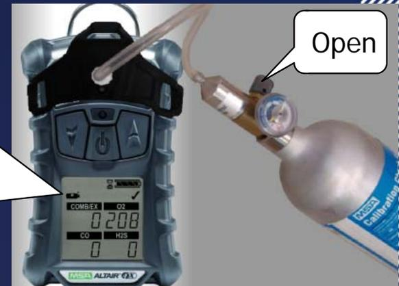
5, "Span Calibration" press central button (YES) to start
